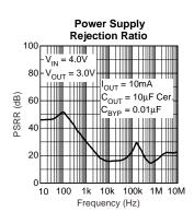
Power Supply Rejection Ratio vs. Voltage
